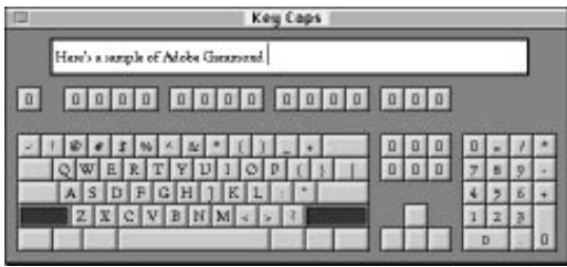
Pressing Shift while in Key Caps displays the Shift versions of the keyboard keys.
